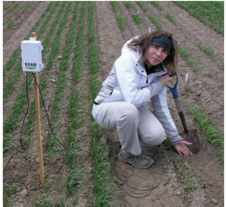
Above, Dr Camille Steber installs Decagon soil moisture sensors. Below, drought trials at Lind Dryland Field Station 2009.
